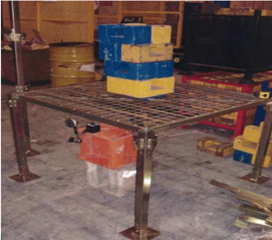
Figure 2-2 Concentrated Load Test (Source: Lloyds British test report)
