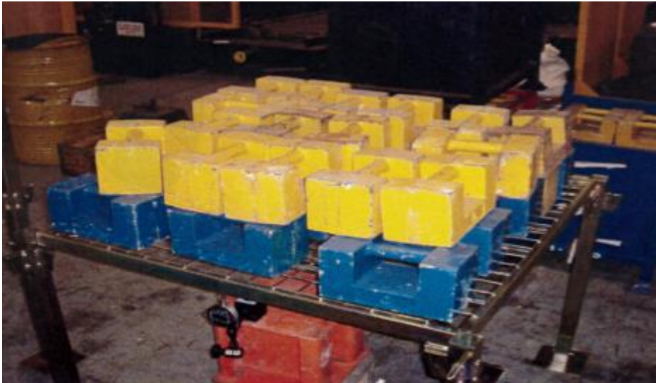
Figure 2-1 Maximum Deflection Test
